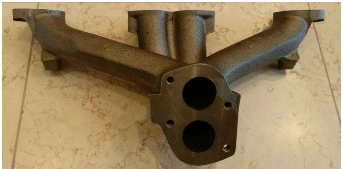
Yugo exhaust manifold and front pipe
