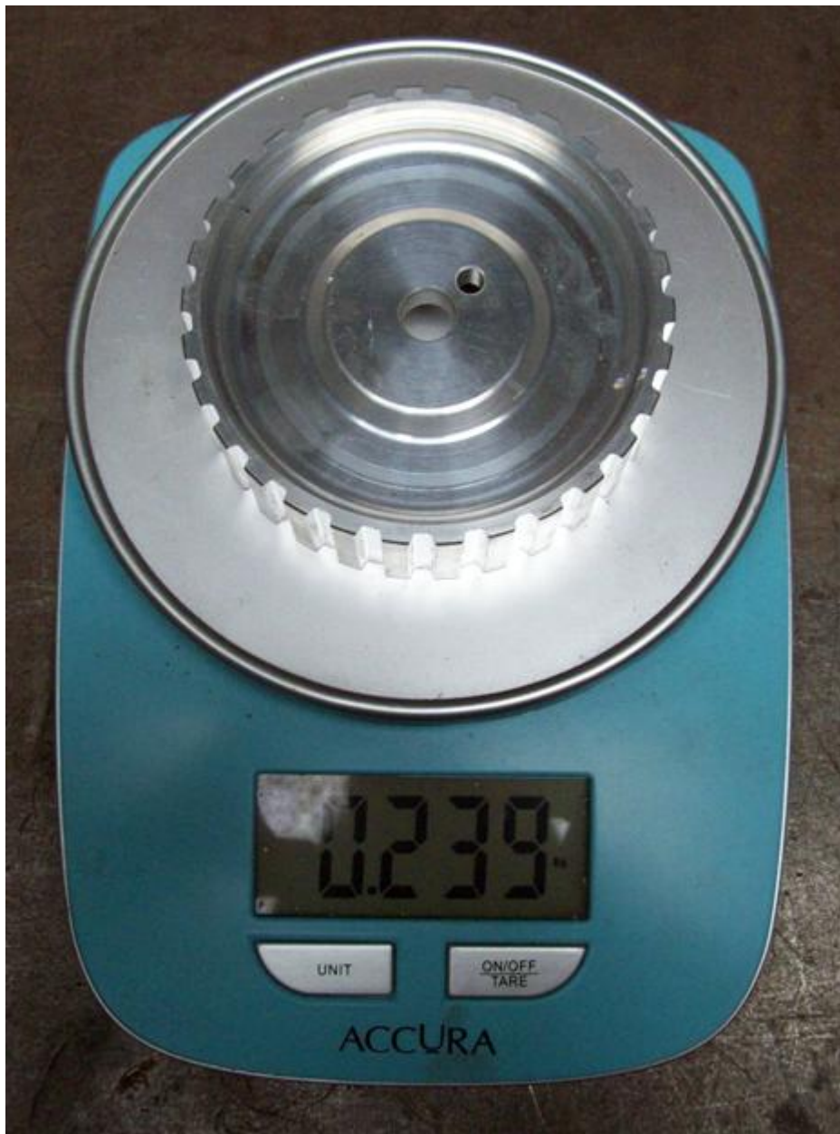
Alquati toothed belt accessory drive crank gear
