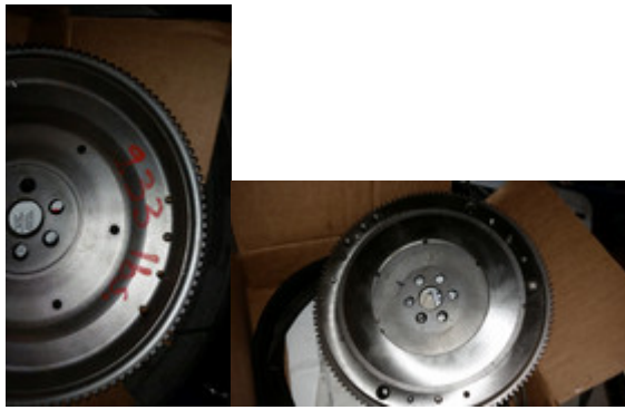
Detail of weight removal 1300 4 speed OE flywheel
