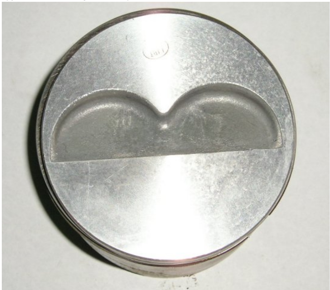
Type 2. Cast in Large valve flycut.
