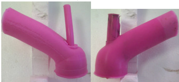
Exhaust / centre of cylinder side of standard and modified ports.
