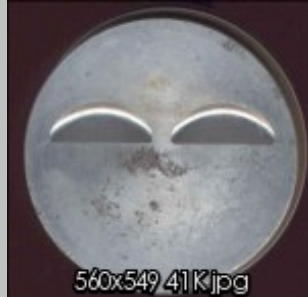
Type 3. machined in small flycut.
