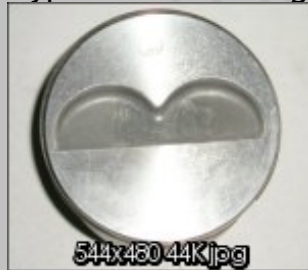
Type 2. Cast in Large valve flycut.
