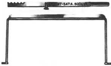
A.60041/2 Valve leak test tools
