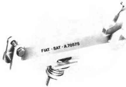
A.70575 Support used in conjunction with hydraulic jack when removing or replacing transmission unit
