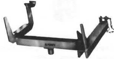
A.70577 Support for removing and refitting power unit - Use with hydraulic jack
