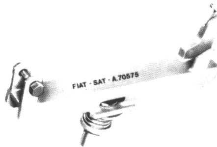
A.70575 Support used in conjunction with hydraulic jack when removing or replacing transmission unit
