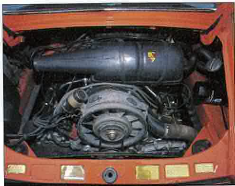
Porsche's classic flat-six (above) powers the 911 Targa. Left-hand drive car is Californian import.
