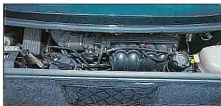
Fuel-injected K-series engine lurks behind this panel in the middle of the MGF.
