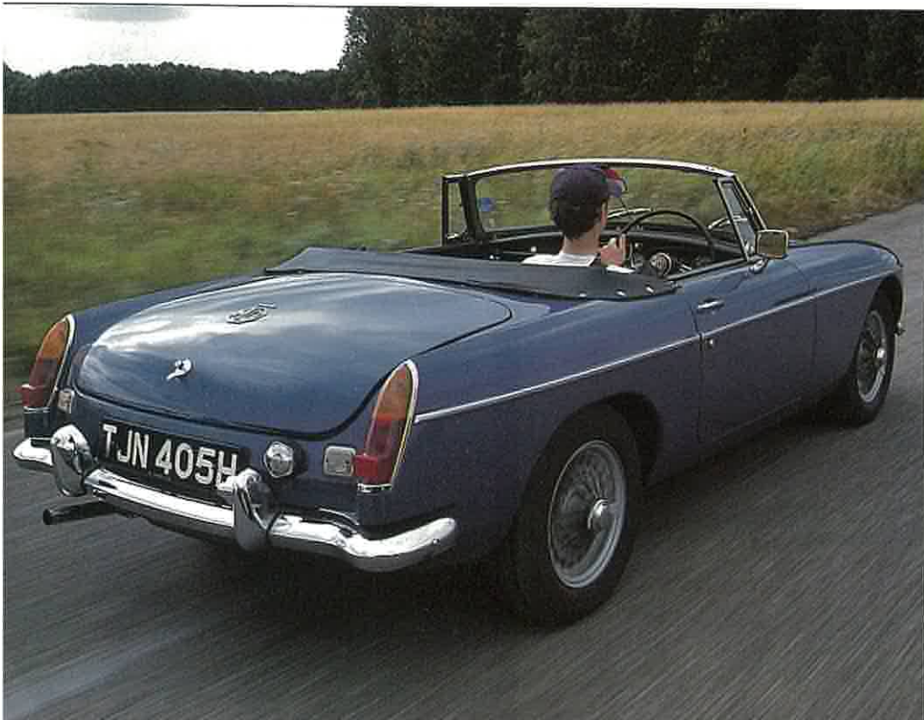
Above: MGB features 1.8-litre B-series engine running twin SUs – classic stuff.
