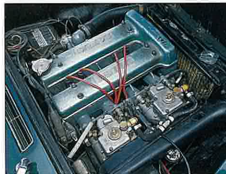
Above: Lotus twin cam fills the Elan's engine bay - there's not a lot of spare room in there!
