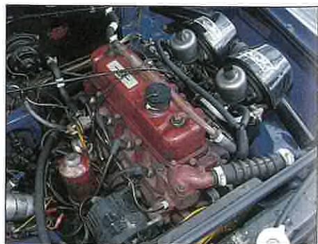
Above: MGB features 1.8-litre B-series engine running twin SUs – classic stuff.
