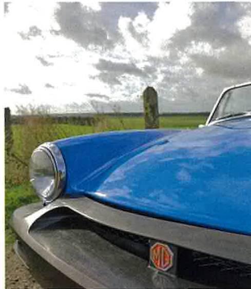
The rubber bumpers were added to meet US safety laws, but the facelift also boosted sales
