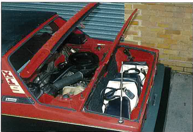
Above: Two compartments in rear, engine then small boot Below: Car boasts useful extra luggage compartment up front.
